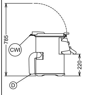
CWI1 = D = Cold Water inlet 1 Drain
